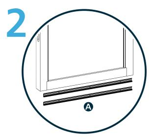
Measure the distance between the parting beads on the window and cut two lengths of Meeting Rail Interlock (A) to fit comfortably without touching the parting beads.
