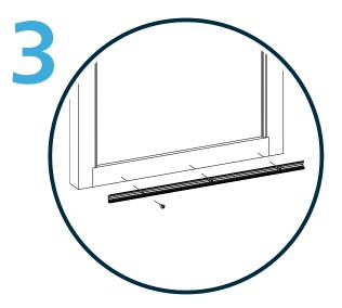
Attach Meeting Rail Interlock (A) onto the first sash using self drilling screws.
