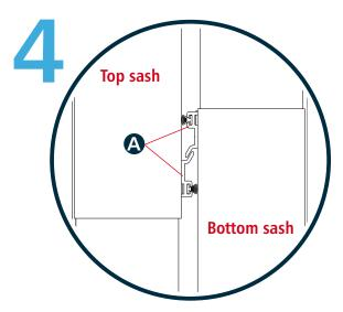
Position and attach the second Meeting Rail Interlock (A) onto the second sash so that the two meeting rails interlock when the window is closed.
