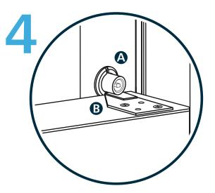
Activate Locking Ventlock **(A)** using the Key **(C)** provided. Lower the sash and install the Strike Plate **(B)**.
