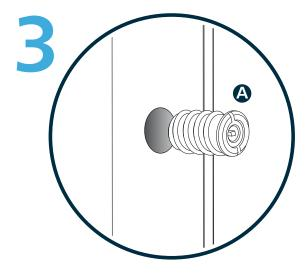
De-activate Locking Ventlock **(A)** using the Key **(C)** provided. Screw the Locking Ventlock **(A)** into the hole using a large flat bladed screwdriver or one of our insertion tools, part code:
