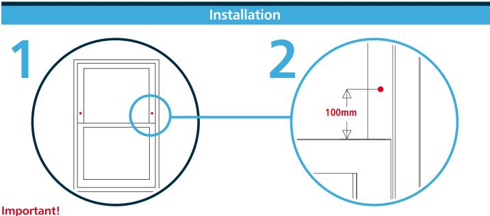
Close and lock sash before starting installation.
