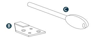
**Important:** Consideration should be given before fitting to Egress windows. Locking Ventlock projects 9mm when fully out. This device must be fitted in a position that allows no more than a 100mm restricted opening. Ensure the sash is completely closed and locked before starting the installation.
