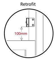
Devices are supplied in pairs and both must be fitted to ensure window is safely secured. One device is fitted to each side of the top sash.
