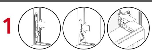
Push top to re-engage window opening control device.
